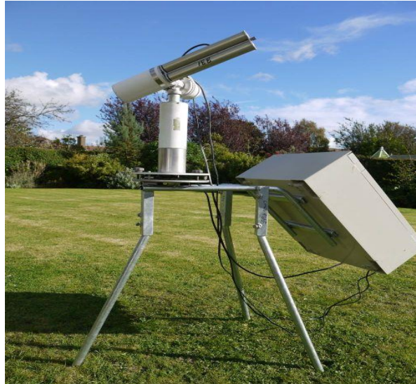
Figure 2.9 The CE 318 automatic sun tracking photometer has been designed and realized to be a very accurate sun photometer with all the qualities of a field instrument ( http://fsf.nerc.ac.uk/instruments/Cimel.shtml ).
