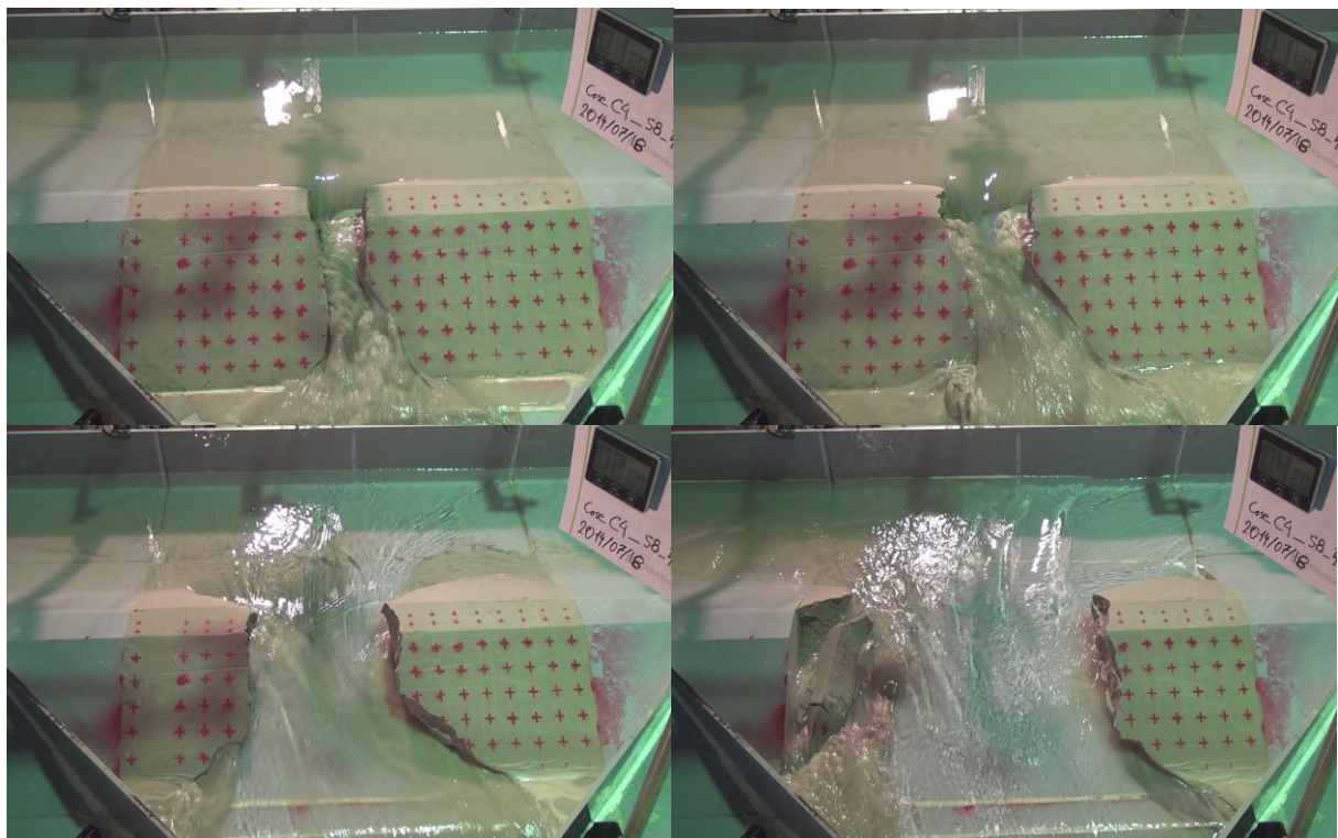
Figure 4.4 Four phases of lateral widening process (Top left-1, Top right-2, Bottom left-3 and bottom right-4)
