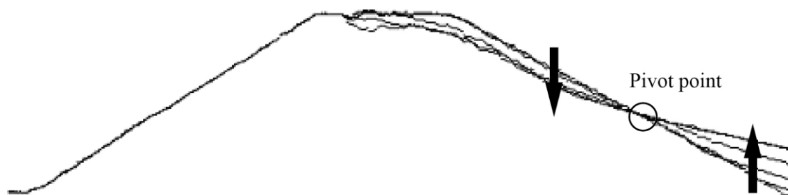
Figure 1.12 Rotation of downstream dyke face around pivot point in the first stage after overtopping (Dupont et al. 2007)
