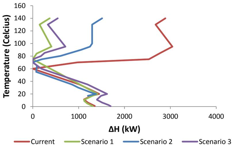
Fig 5.7: The GCC obtained from pinch analysis of current mushroom processing (red), Scenario 1 (Slicing before vacuum hydration, green) Scenario 2 (vacuum hydration with hot water, blue) and Scenario 3 (vacuum hydration with blanch water, purple).
