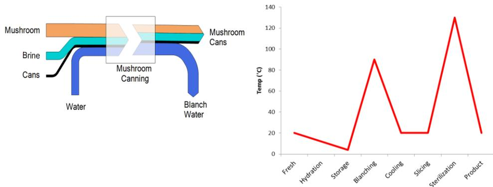
*Fig 1.4: **Left:** Mass balance of canned mushroom production shown with Sankey diagram. **Right:** Temperature change in mushroom at various unit operations.*
