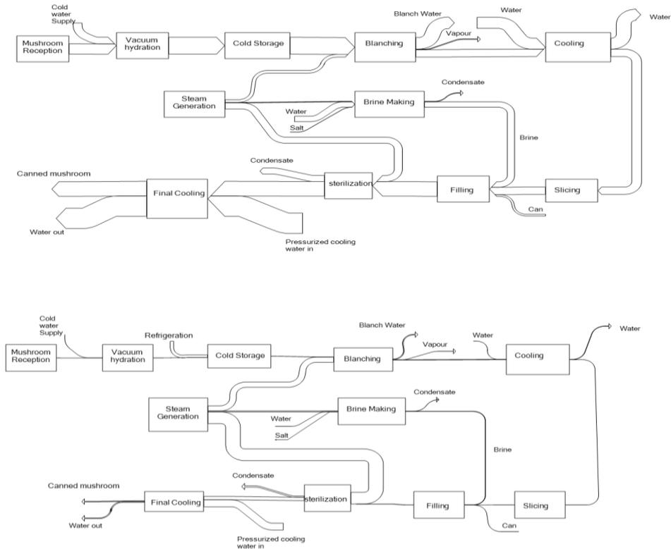
Fig 5.2: The Sankey diagram of mass (top) and physical exergy (bottom) flow of the current canned mushroom production system. The widths of the arrows show the size of the mass or exergy of the streams. In the exergy Sankey, also called Grassmann diagram, the difference between the ingoing and outgoing arrows for any
