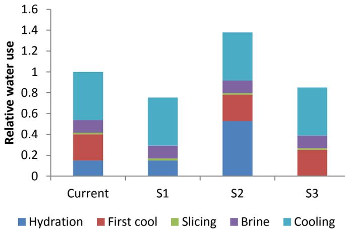
*Fig 5.9: Relative water requirement for various unit operations compared to the total water requirement of the current process.*
