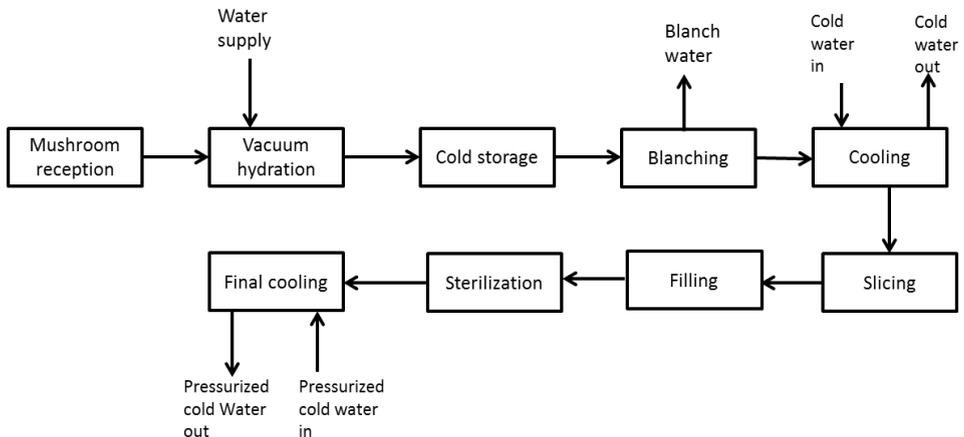
*Fig 1.3: The block diagram of mushroom flow in canned mushroom production*
