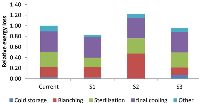
Figure 5.10: Relative exergy losses of various unit operations compared to a total exergy loss in current processing for various scenarios
