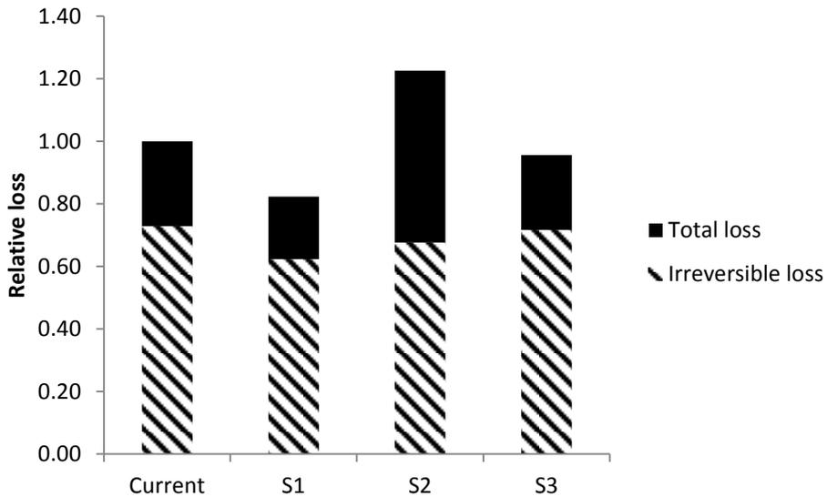
Fig 11: Irreversible exergy loss (stripped lower ) shown as a fraction to total exergy loss in current production
