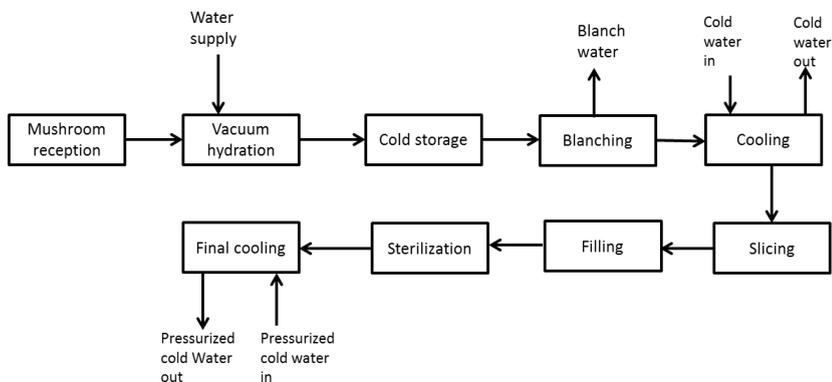
Fig 5.1: Schematic flow diagram of the current production of canned mushrooms
