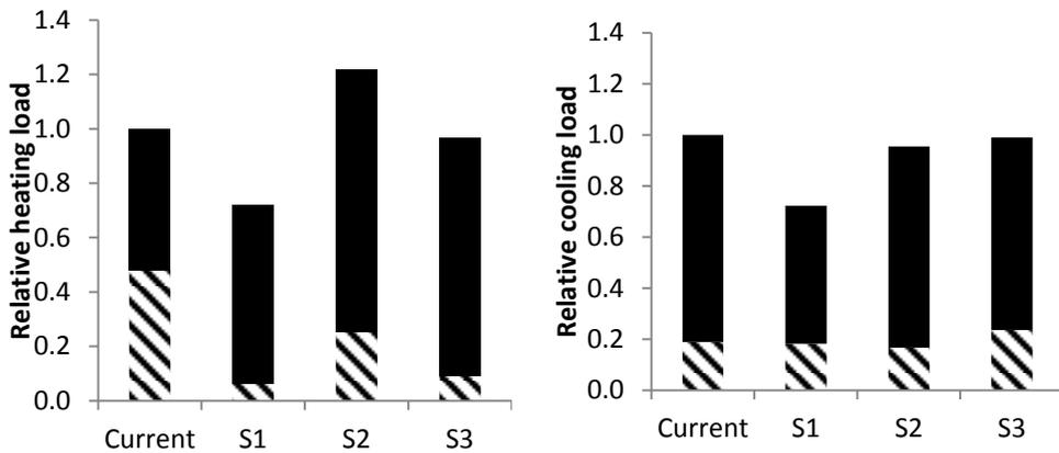
*Fig 5.8: The heating and cooling requirement of different scenarios as the fraction of those requirements in the current process. The patterned lower part of the graph shows external utility requirements under the pinch (i.e., the lowest possible heating or cooling load necessary).*
