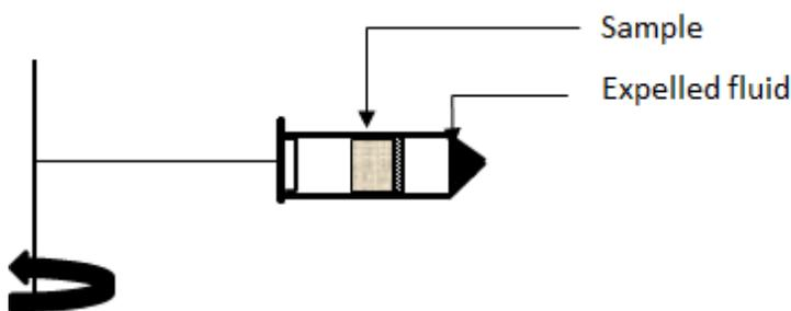
Fig 2.1: An illustration of application of centrifugal force in the mushroom sample.
