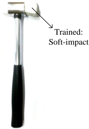
Figure 5.3 Impact hammer with soft rubber used for reference database construction.
