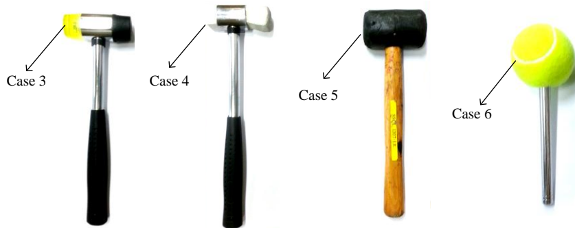
Figure 5.13 Impact hammer with large contact area.
