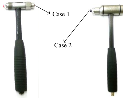
Figure 5.12 Impact hammer with small contact area.
