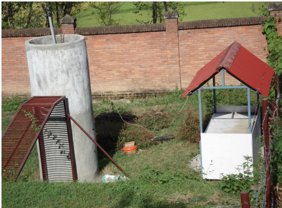
Photograph 4: Lysimeter and Temperature Probe
