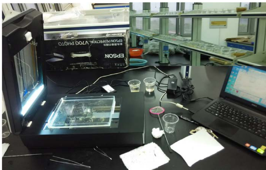
Figure 5.3 Root scanning with EPSON V700 flatbed scanner
