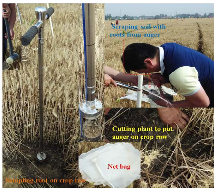
Figure 5.1 Root sampling by root auger and transferring it to net bag
