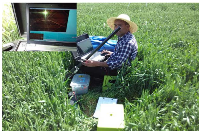
Figure 5.5 Non-destructive root measurement by WinRHIZO TRON
