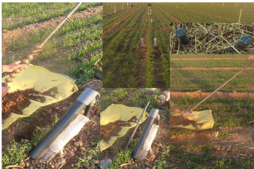
Figure 5.4 Installation of Mini WinRHIZO TRON tube
