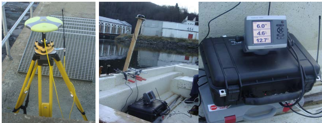
Figure 2-5: Base station Transducer and GPS and fitted on boat and GARMIN Fish Finder at Øvre Leirfoss
