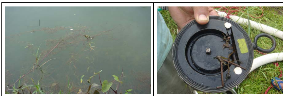
Figure 7-9: Dense weed growth in the peaking pond and debris catching on the check valve plate.
