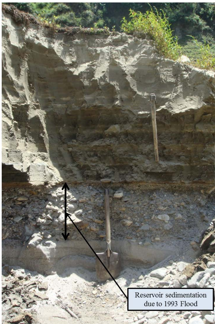
Figure 4-20: Sediment deposition layers in the Kulekhani reservoir (For location, see Figure 4-14)
