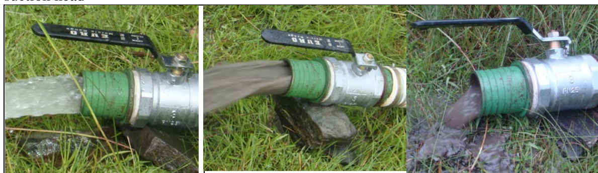
Figure 7-6: Flow at the outlet after priming, normal and clogged flow
