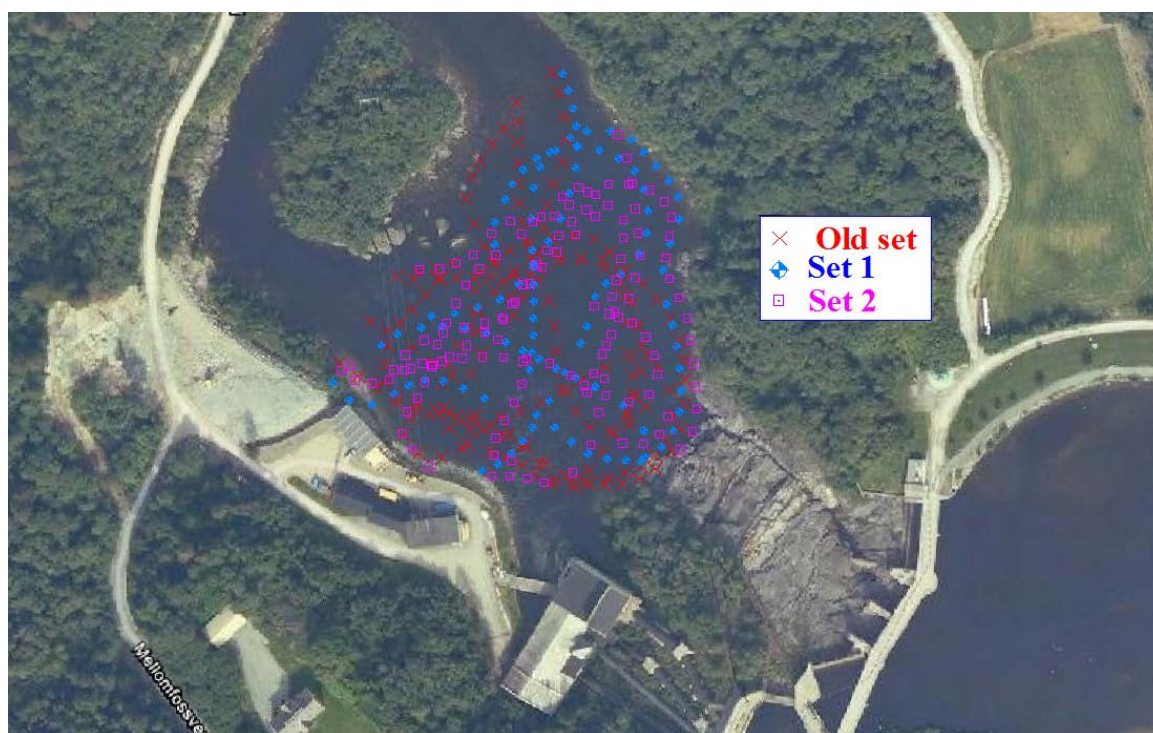
Figure 2-6: Survey track lines and the surveyed area in Øvre Leirfoss (picture from http://kart.gulesider.no/ )
