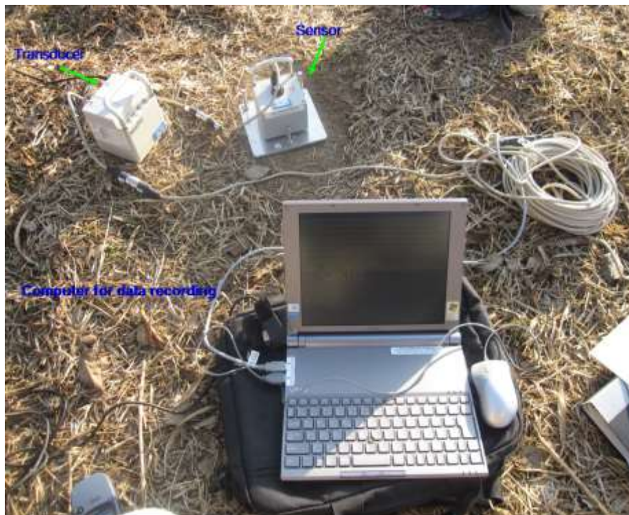
Figure 4.3: Instruments used for the microtremor survey in Kathmandu Valley.
